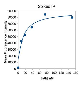
**Spiked IP** Tritration curve of rAb against antigen of interest. The  $K_D$  values were obtained by the least-squares fitting of fluorescence saturation data.
