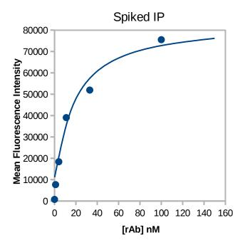
**Spiked IP** Tritration curve of rAb against antigen of interest. The  $K_D$  values were obtained by the least-squares fitting of fluorescence saturation data.
